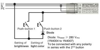
This driver supports single and double button Touch DIM operation. The 2<sup>nd</sup> button must be connected in parallel with the 1<sup>st</sup> by means of a diode. As per factory default configuration, they are used:
